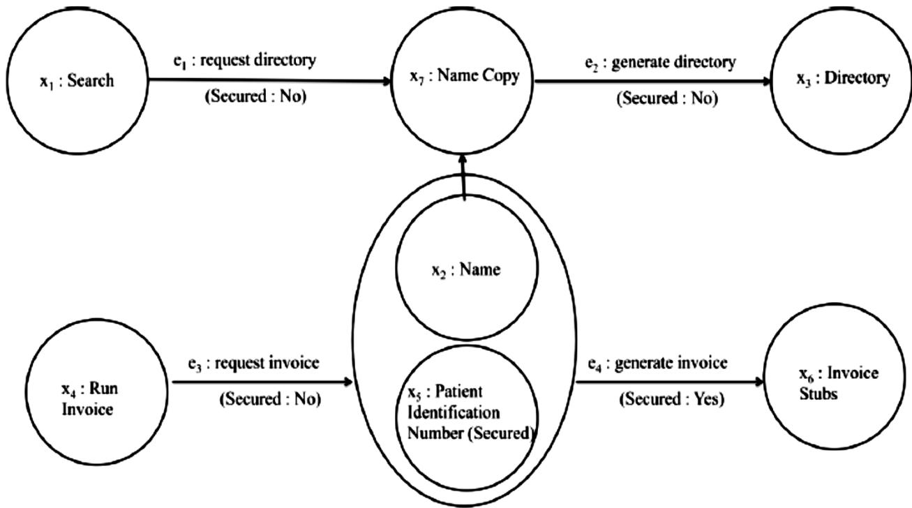
Figure 2. Metagraph of Processes with Layer.
