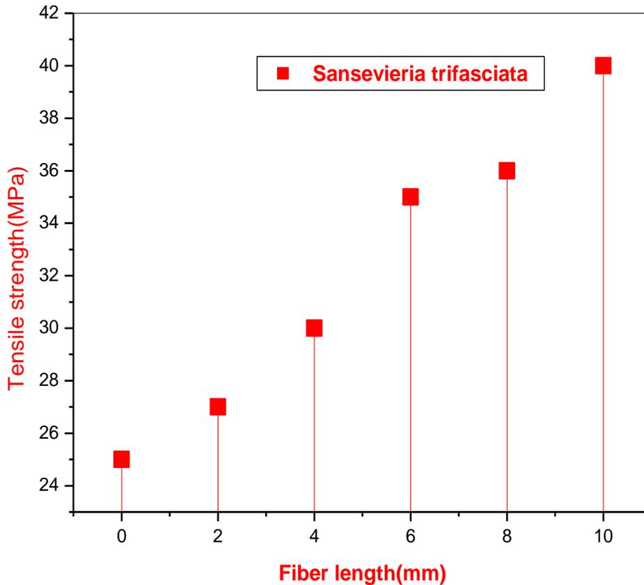
**Figure 1.** Average tensile strength of short *Sansevieria trifasciata* reinforced polyester composite with fiber length.
