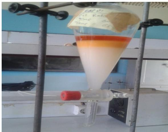
**Fig.6:** Washing of biodiesel
