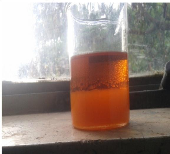
**Fig.5:** Transestrification reaction and biodiesel layer
