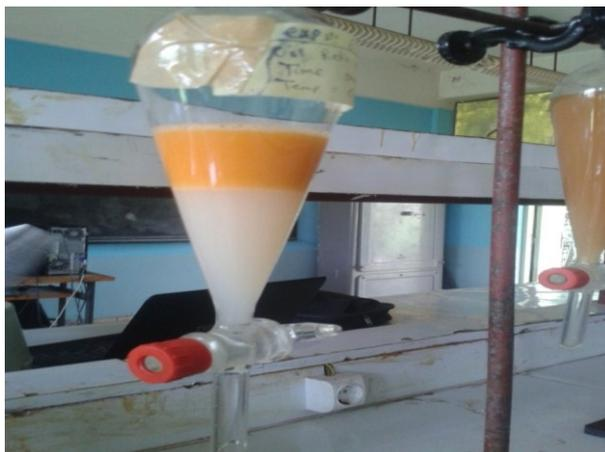
**Fig.8:** Glycerol separation using water
