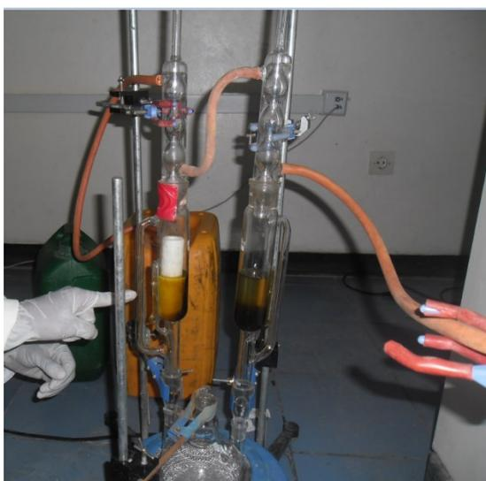
**Figure 1.** Soxhlet apparatus set up.
