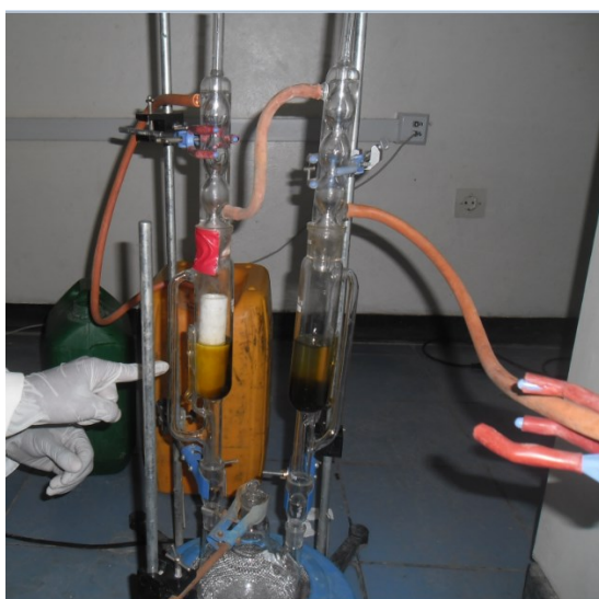
Figure 1. Soxhlet apparatus set up.
