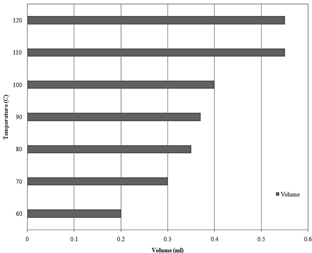
Fig. 4. Effect of temperature on extraction of oil.
