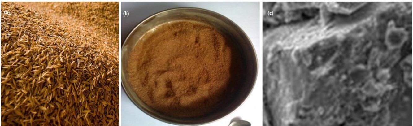
**Fig. 6.** Rice husk (a) raw (b) grinded (c) surface of rice husk.
