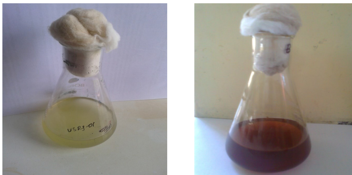
Figure 2. Colour change observed in cell free fungal filtrate of Aspergillus spp after exposure to silver nitrate.
