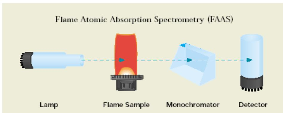
**Fig. 3.**Operational principle of an atomic absorption spectrometer
