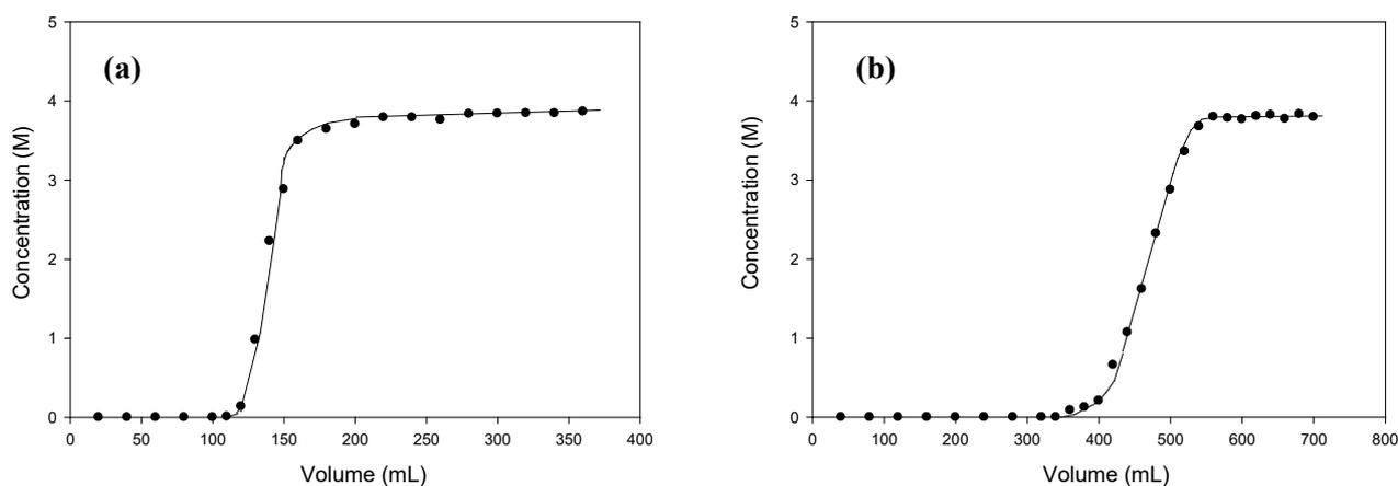
**Figure 5.** Breakthrough curve of (a) sand and (b) sugarcane bagasse.
