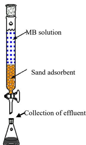
**Figure 3.** Conventional column for continuous column adsorption study.
