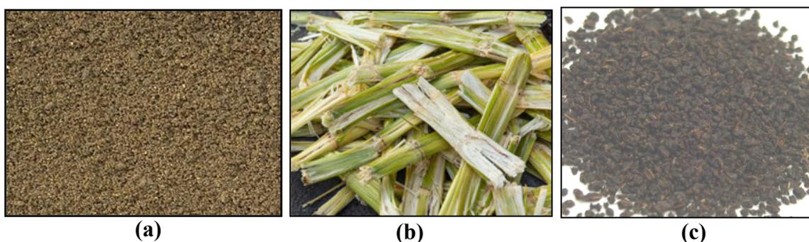
**Figure 1.** Raw materials of adsorbents: (a) sand, (b) sugarcane bagasse and (c) Fresh black tea leaves.
