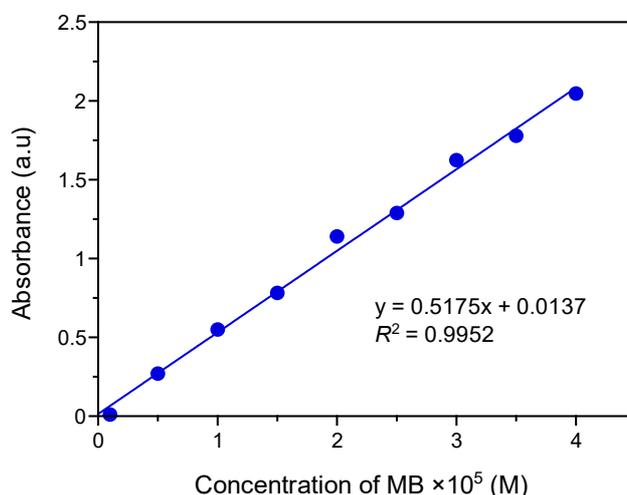
Figure 4. Calibration curve for analysis of Methylene blue.
