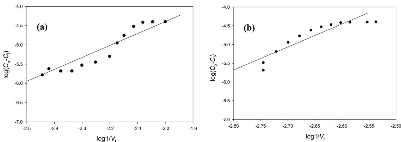
**Figure 7.** Column exhaustion capacity of (a) sand and (b) sugarcane bagasse.
