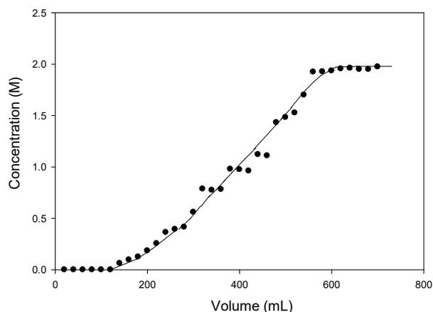
**Figure 6.** Breakthrough curve of used black tea leaves (UBTL).
