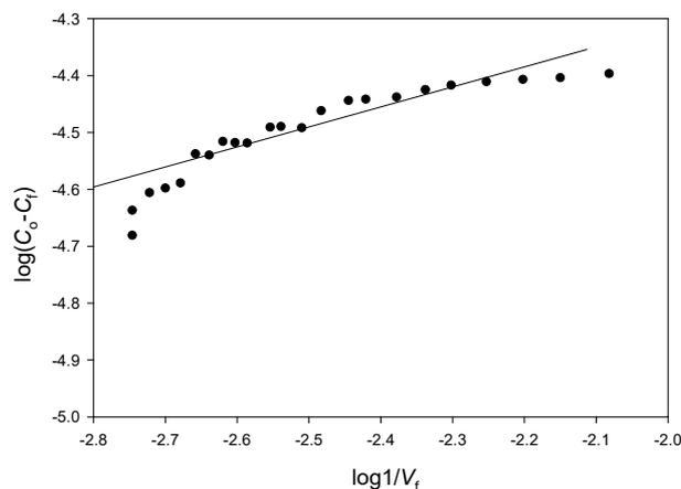
**Figure 8.** Column exhaustion capacity of used black tea leaves (UBTL).
