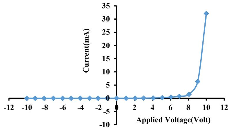
Fig. 9. I-V characteristic under forward and reverse bias of n-CdO-CdO<sub>2</sub>/P-Si at 100 °C.
