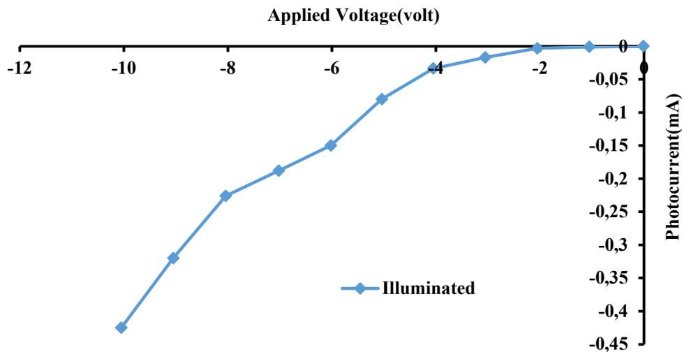
Fig.10: Illuminated (I-V) chara-cteristic of n-CdO-CdO<sub>2</sub>/P-Si solar cell at 100 °C.
