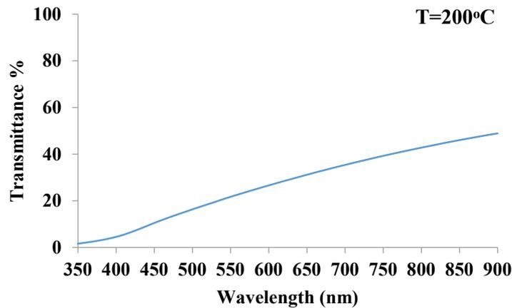
Fig. 4. Transmittance spectrum of CdO-CdO<sub>2</sub> thin films.
