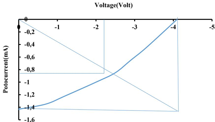
Fig11. I-V characteristics (n-CdO-CdO<sub>2</sub>/p-Si) solar cell at 100 °C.
