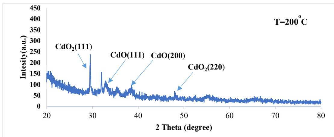
Fig. 2. XRD pattern of CdO-CdO<sub>2</sub> thin films, which prepared by chemical method and deposited by drop casting technique on glass at Annealing temperature of 200<sup>0</sup>C.
