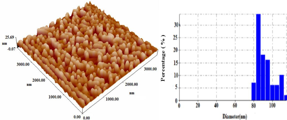
Fig. 3. 3D AFM images of CdO-CdO<sub>2</sub> thin film surface and Granularity accumulation distribution chart at Annealing 200°C.
