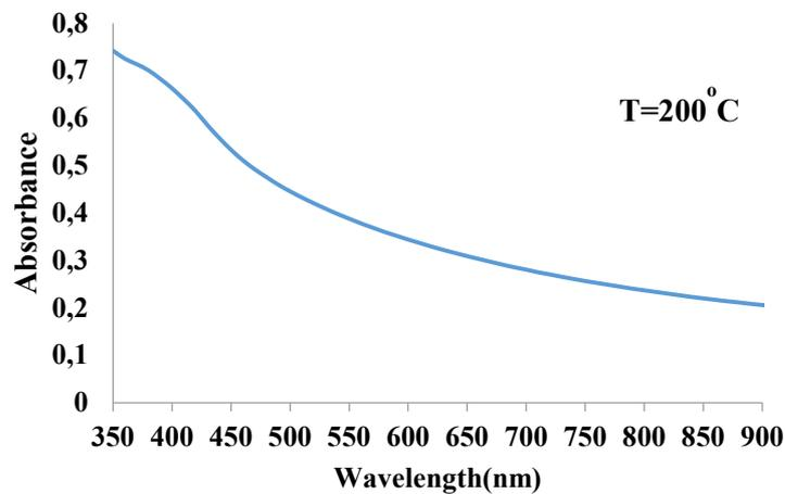
Fig. 5. Absorbance of the as deposited CdO-CdO<sub>2</sub> thin films.
