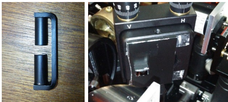
Figure 3. (left) Photo of the neodymium magnets attached to the yoke. (right) Photo of the InAs emitter attached to the magnet holder.
