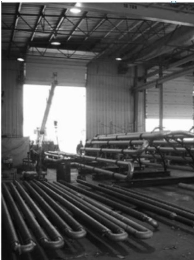
**Figure 2:** Heat transfer coils for refinery heaters showing a coil for cabin heater (foreground) and cylindrical heater in the background (photos provided courtesy of Born Heaters, Canada, an Onquest Company)
