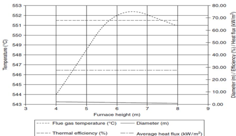
**Figure 4:** Effect of furnace height on principal parameters in the design of a cylindrical oil heating furnace
