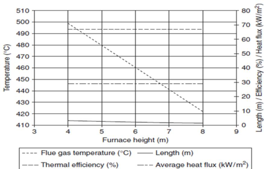
**Figure 3:** Effect of furnace height on principal parameters in the design of a rectangular oil heating furnace
