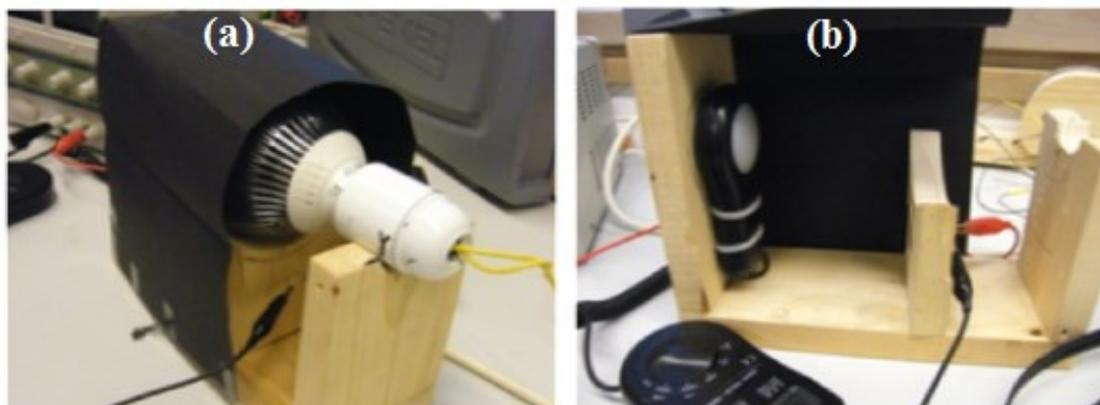
**Figure 2.** Light measuring setup (a) outer look of the setup, (b) inside view of the setup.
