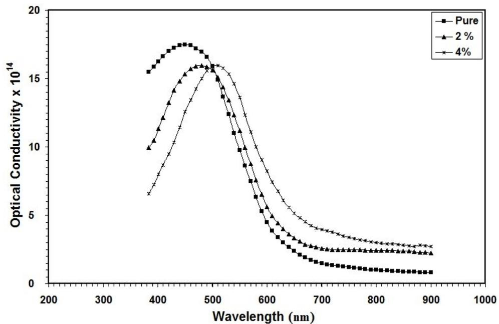
Fig. 5. Plot of optical conductivity vs wavelength of Cu:NiO thin film.
