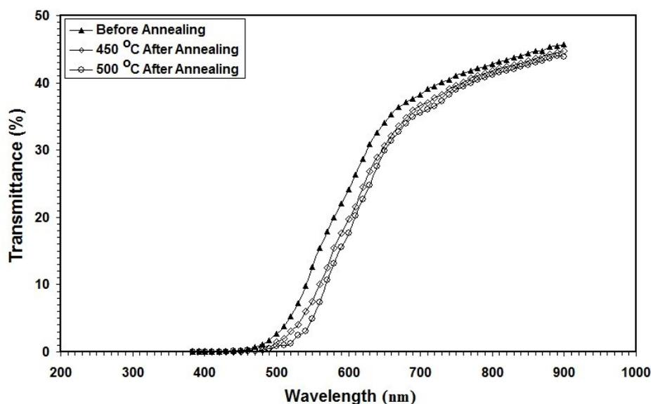
Fig. 1. The transmittance spectra versus wavelength of Cu:NiO thin film.
