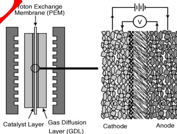
**Figure 5.** Membrane-electrode assembly of typical PEM URFC.
