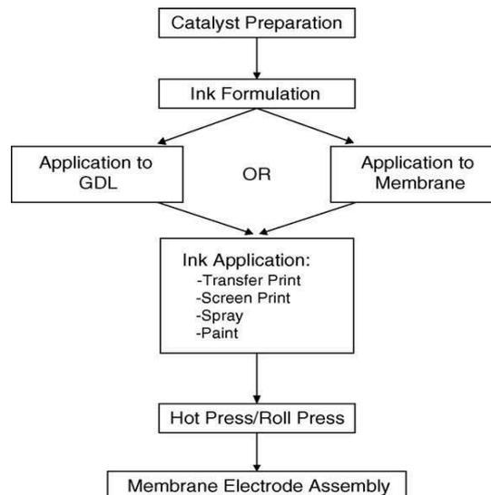
**Figure 8.** Flow diagram of URFC MEA assembly
