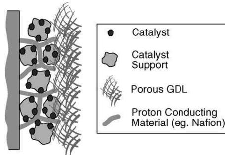
**Figure 7.** Schematic of typical URFC membrane-electrode interface
