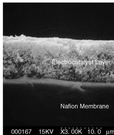
**Figure 3.** Scanning electron micrograph (SEM) of a cross-section of an electrocatalyst assembly.
