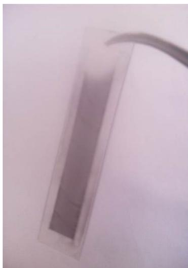
**Figure 3.** Polyoyrrole film synthesised in lyotropic liquid crystal.
