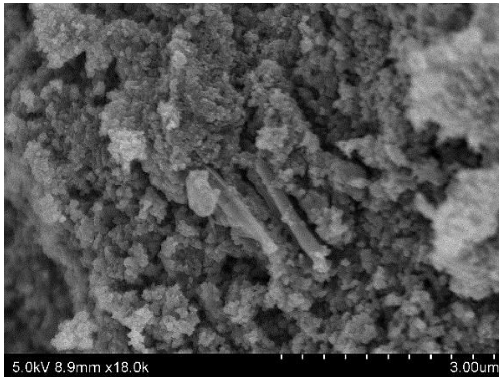
Fig. 3. SEM image of DSSC photoanode fabricated from mixed TiO 2 nanorods/ nanoparticles (5:95 by mass fraction).
