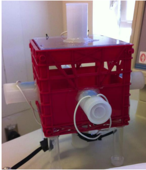
Figure 2. Smaller “4-D” application geometry showing the 3 pairs of solenoids (reed relays) that generate the magnetic fields within each plane successively and then in all planes simultaneously. Malignant cells within the effective zone (~10.6 cm diameter) produced by this spatial rotation exhibit dissolution as indicated by their absence. Inside width of box is 14 cm. Note the exposures occur in complete darkness within the incubators.
