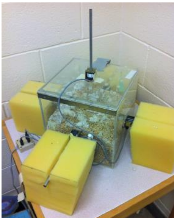
Figure 1. Picture of the “4-D” exposure equipment that generates “spatially” rotating frequency and phase-modulated magnetic fields through successive spatial planes and then in all planes simultaneously that is driven by optocouplers within an electronic circuit.
