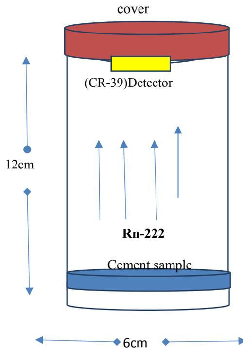
**Fig. 1.** A schematic diagram of the sealed-cup technique.
