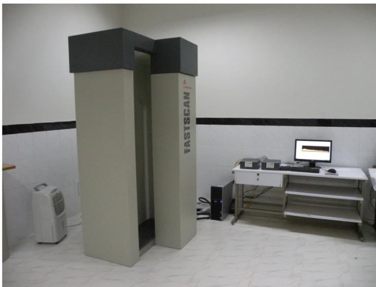
Figure 1. CANBERRA FASTSCAN Whole Body counting arrangement (model 2250).
