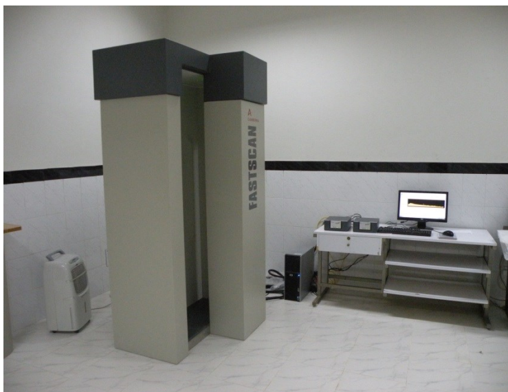
Figure 1. CANBERRA FASTSCAN Whole Body counting arrangement (model 2250).
