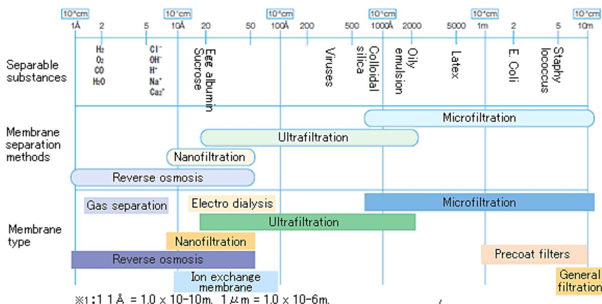
Figure 2. Classification of various membrane separation processes [19].
