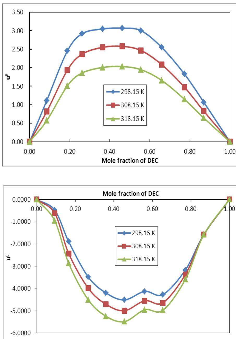
**Figure 3.** Variation of Excess speed of sound ( $u^E$ ) with mole fraction of diethyl carbonate for (a) diethyl carbonate + benzonitrile and (b) diethyl carbonate + benzaldehyde system at different temperatures.
