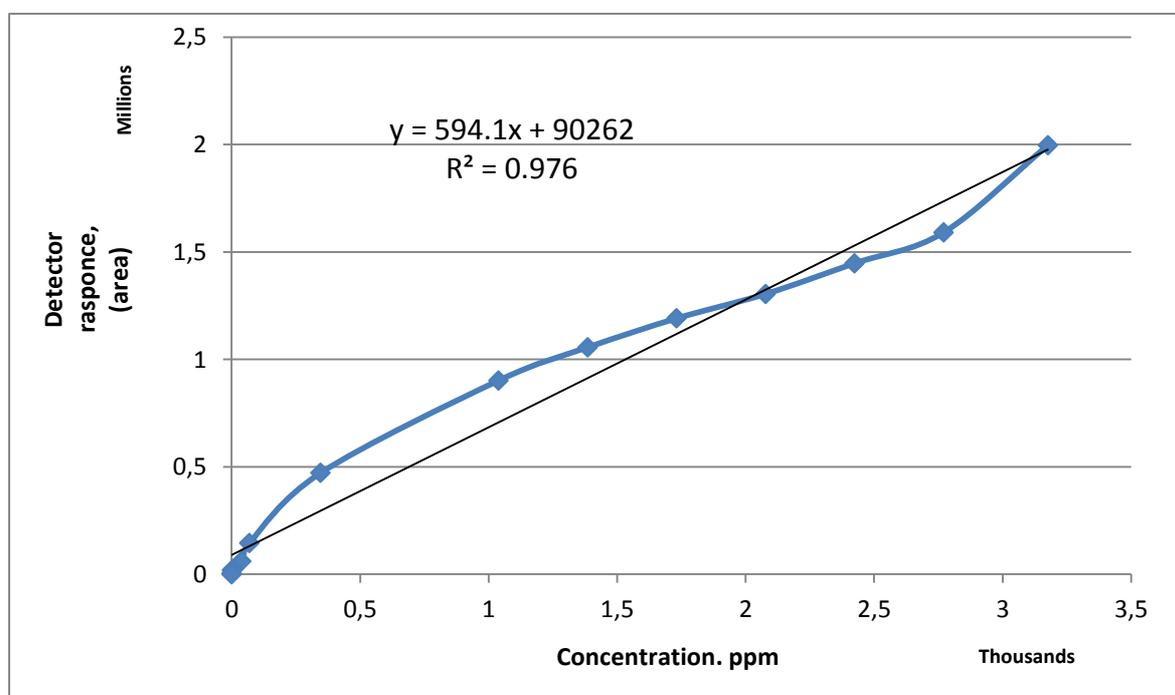
Fig. 11. Linear range of the detector (FPD-P-mode) for Malathion measured at optimum operating conditions.
