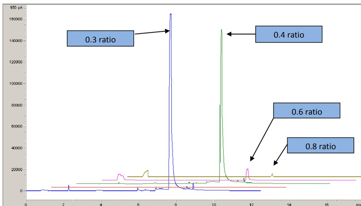
**Fig. 6.** 3D chromatograms of different air to H<sub>2</sub> ratio GC-FPD-P mode for Dimethoate, measured at GC operating condition.
