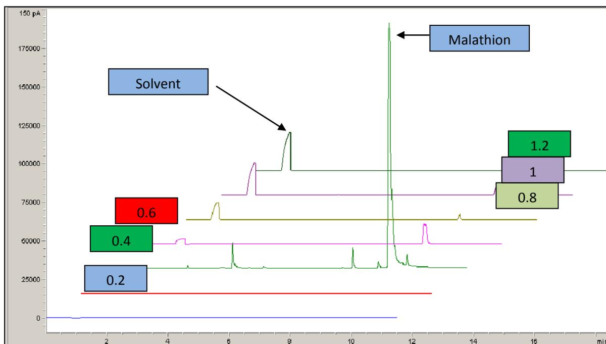
**Fig. 5.** 3D chromatograms of different air to H<sub>2</sub> ratio GC-FPD-P mode for Malathion, measured at GC operating condition.
