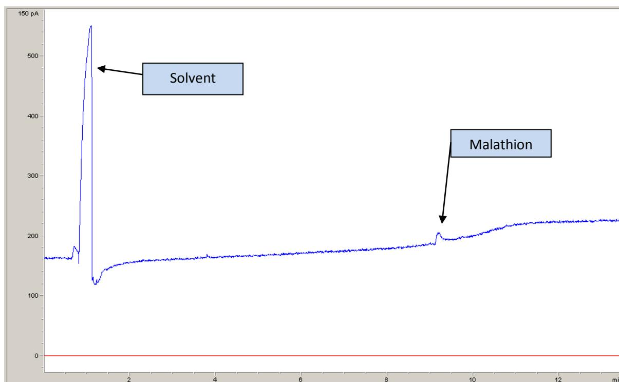
**Fig. 13.** Chromatogram of  $1.88 \times 10^{-3}$  mg/l Malathion (LOD), at optimized conditions.
