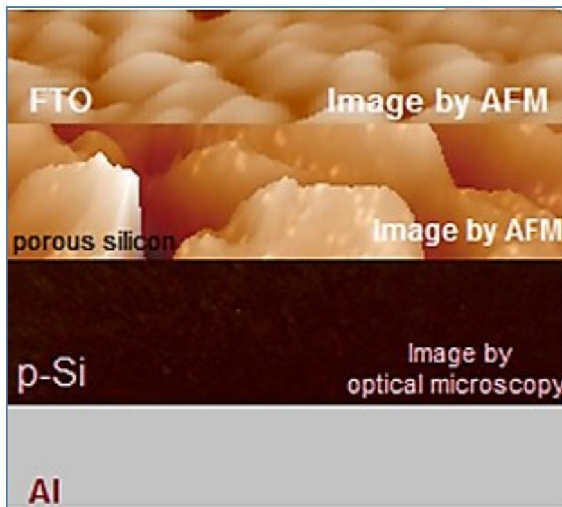
**Figure 2.** A schematic diagram of the FTO/PS/p-Si/Al/ heterojunction.
