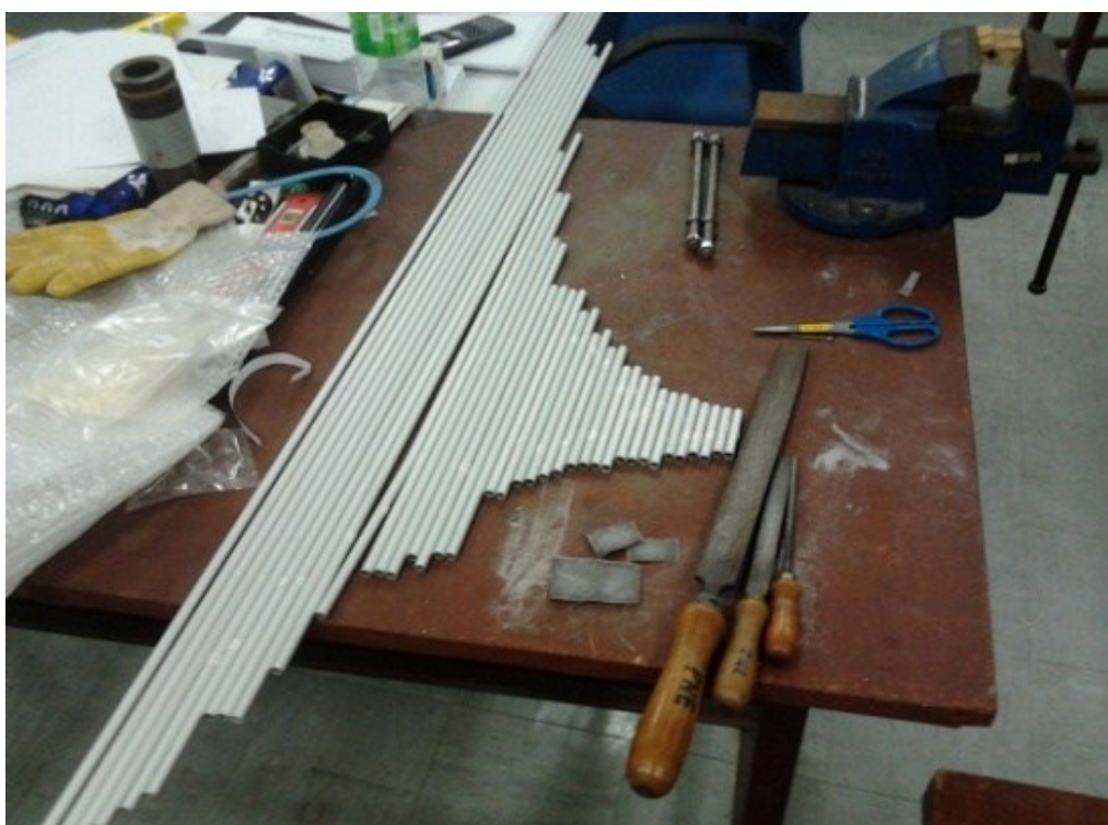
Figure 1. Preparation of construction of LPDA.
