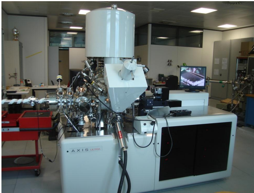
Fig. 6. View on XPS instrument used for the study of surface film formed after EP and MEP.
