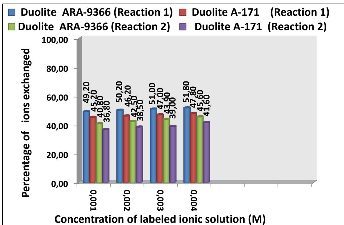
**Figure 2.** Variation in Percentage Ions Exchanged with Concentration of Labeled Ionic Solution.
