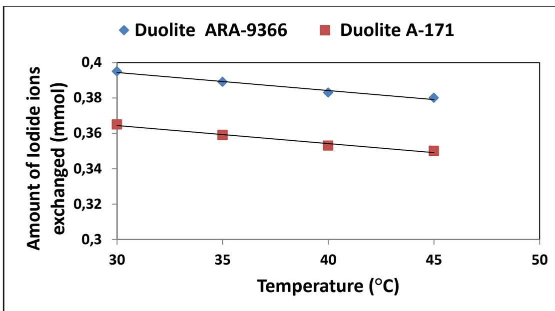
**Figure 6.** Correlation between Temperature of exchanging medium and amount of iodide ion exchanged.
