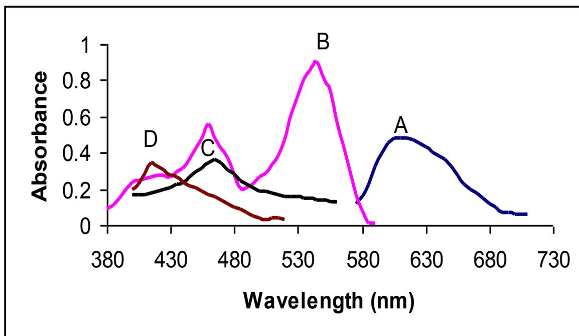
**Fig. 2.** Absorption spectra of: *A*) Green colored manganate ion ( $\lambda_{\text{max}}$  610 nm), *B*) red colored SFS-Cu(II)-eosin ternary complex ( $\lambda_{\text{max}}$  545 nm), *C*) Reddish yellow colored SFS-Mo(SCN)<sub>6</sub><sup>-</sup> ternary complex ( $\lambda_{\text{max}}$  465 nm), *D*) Yellow colored SFS-bromocresol green ion-pair complex ( $\lambda_{\text{max}}$  415 nm)
