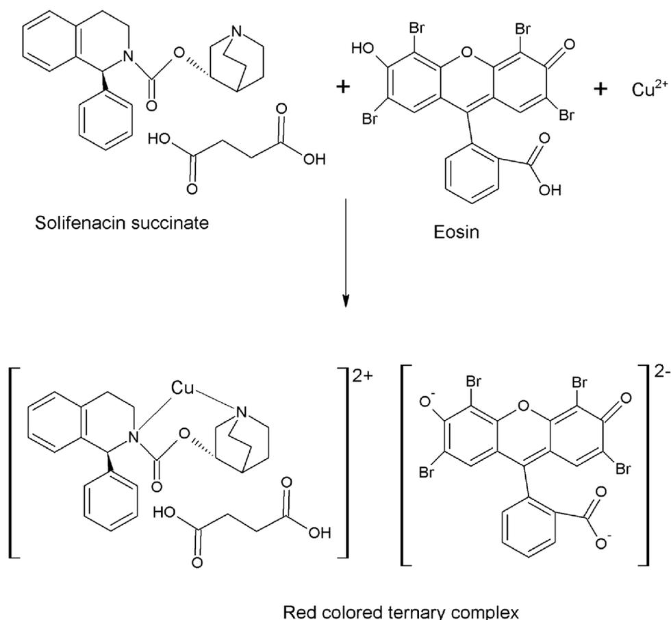
**Fig. 3.** Proposed reaction mechanism for the formation of SFS-Cu(II)-Eosin ternary complex.
