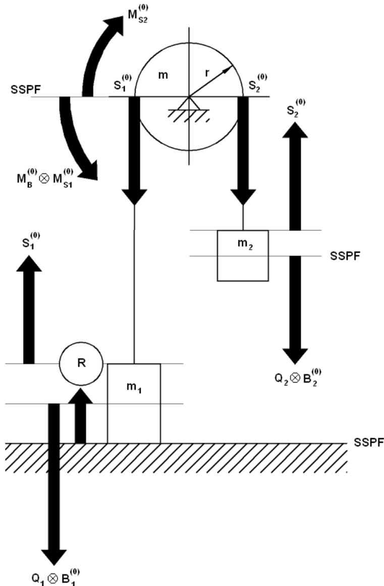
**Fig. 3.** Conditions of stable static energetic equilibrium of elements in the Atwood device.
