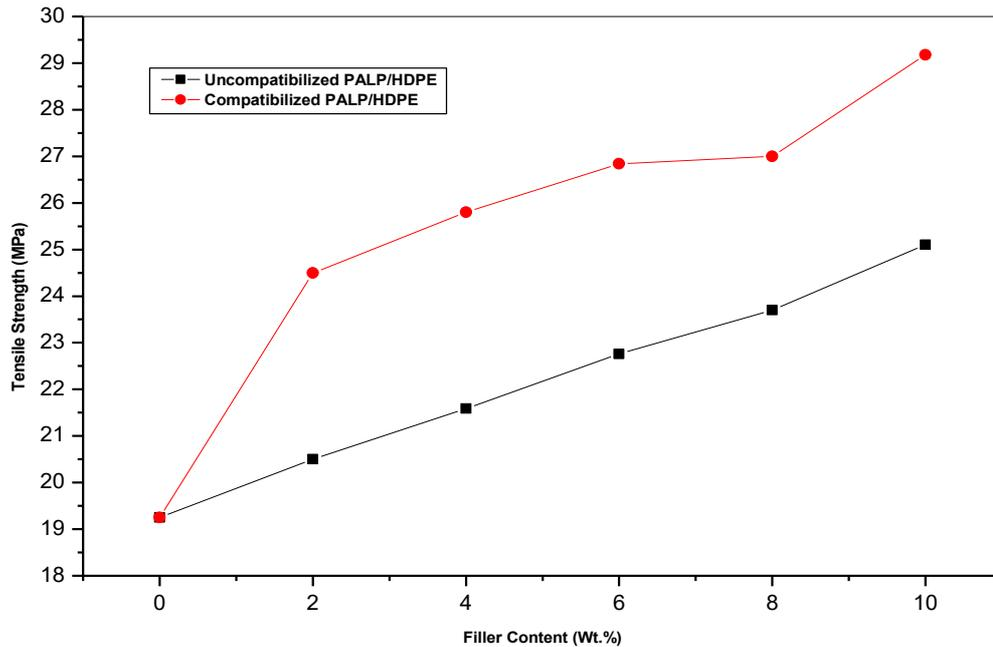
**Figure 3.1.** Effect of Compatibilizer on the Tensile Strength of composites.
