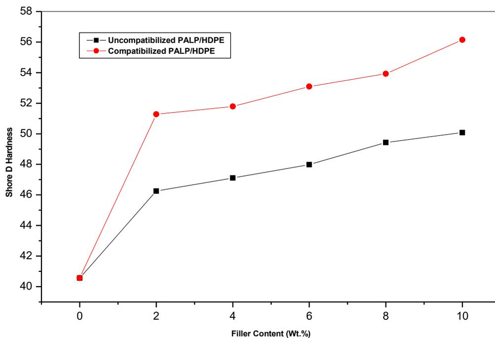
**Figure 3.5.** Effect of Compatibilizer on the Hardness of Composites.
