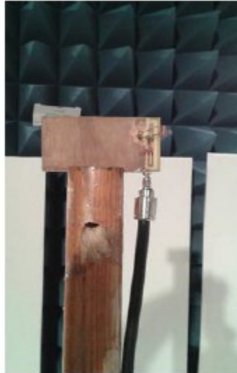
Figure 11. Designed antenna into anechoic chamber.
