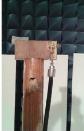
Figure 11. Designed antenna into anechoic chamber.
