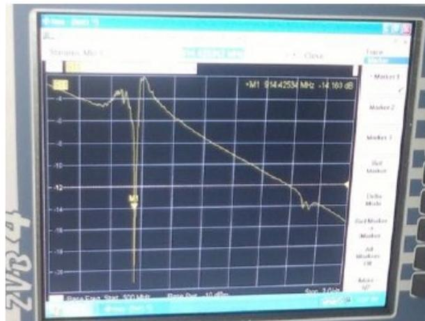
Figure 9. Magnitude vs. Frequency (S<sub>11</sub> Parameter).
