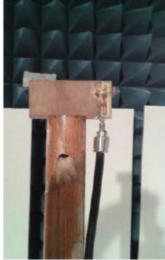
Figure 11. Designed antenna into anechoic chamber.
